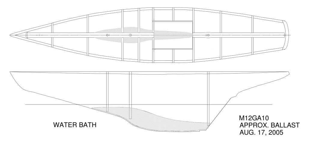
CASTING LEAD BALLAST IS NOT RECOMMEND FOR HEALTH AND SAFETY REASONS AND MAKES BALANCING THE BOAT DIFFICULT. AN INITIAL BATCH OF ABOUT 7 LBS. OF LEAD SHOT MIXED WITH EPOXY CAN BE POURED INTO THE HULL AND ADJUSTED FOR LEVEL OR SLIGHTLY BOW DOWN BALANCE. WHEN BOAT IS FULLY RIGGED A FINAL AMOUNT MAY BE ADDED TO BRING BOAT UP TO MINIMUM 16 LBS. WATER BATH FOR BALANCING AND FOR COOLING WHILE EPOXY CURES.
